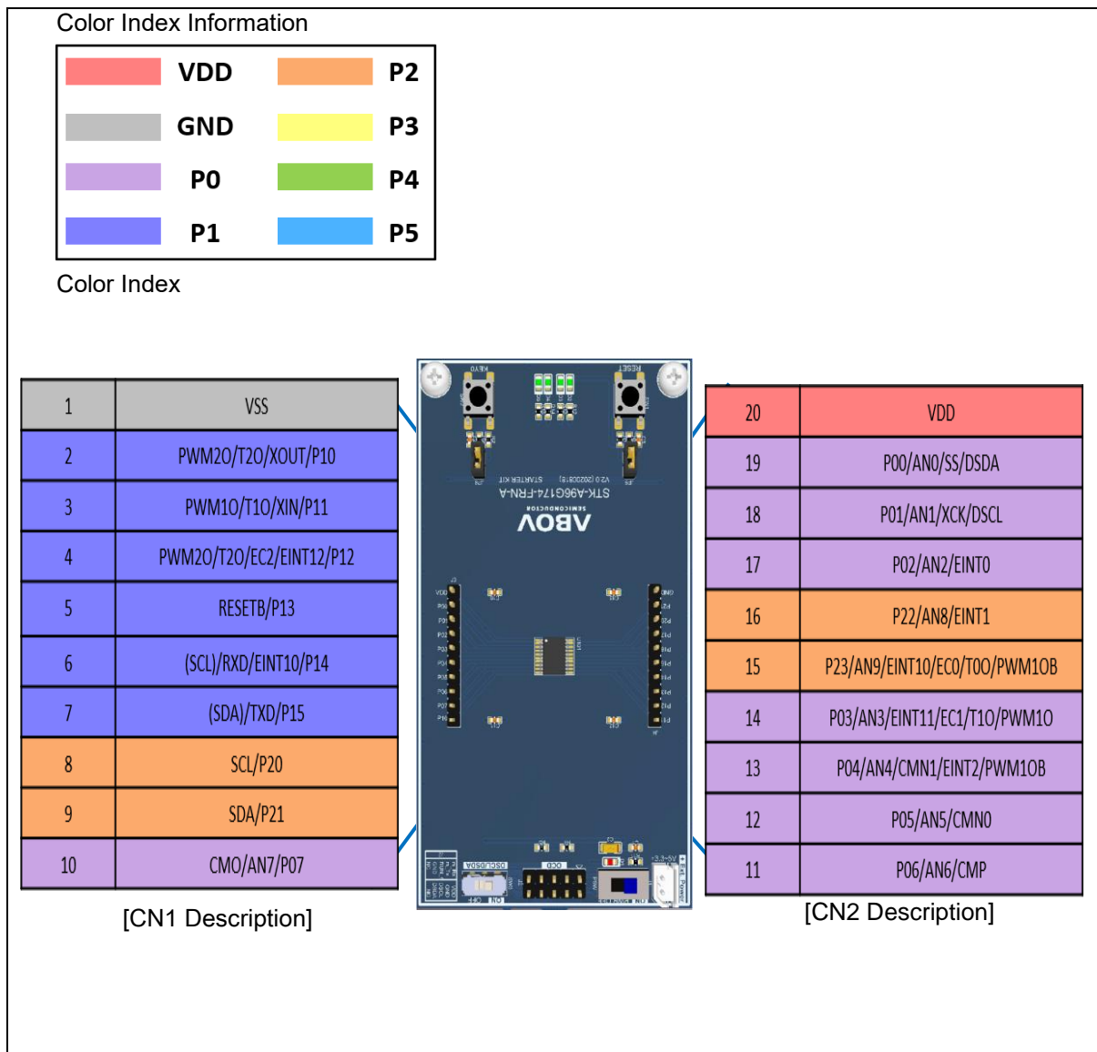
Figure 6. Pin Header
