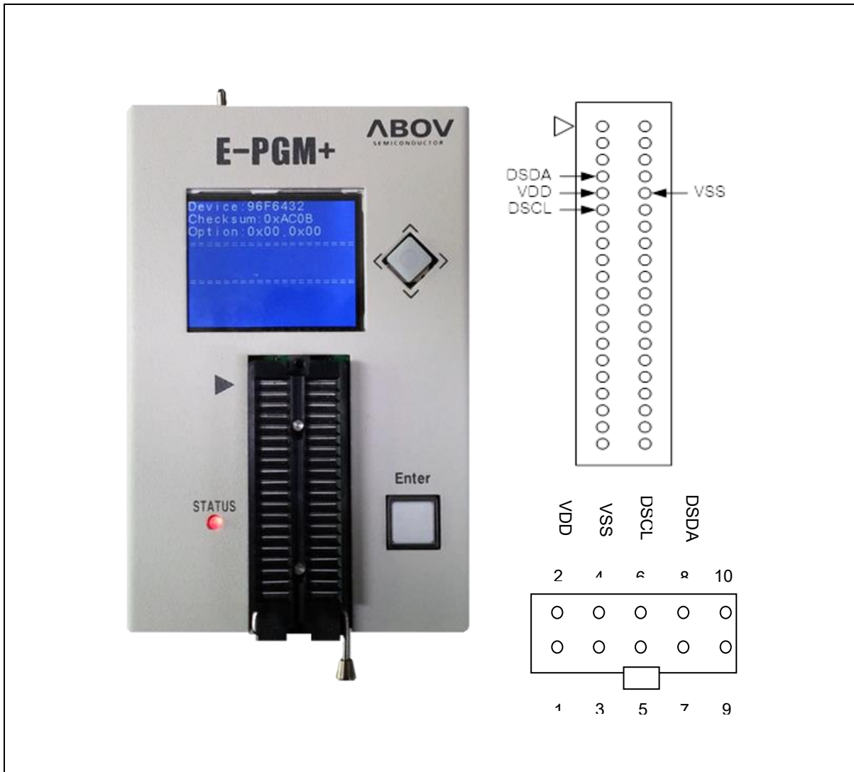
Figure 116. E-PGM+ (Single Writer) and Pinouts
