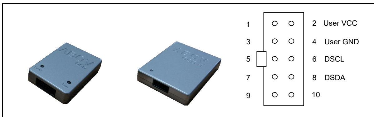
Figure 110. Debugger (OCD1/OCD2) and Pinouts
