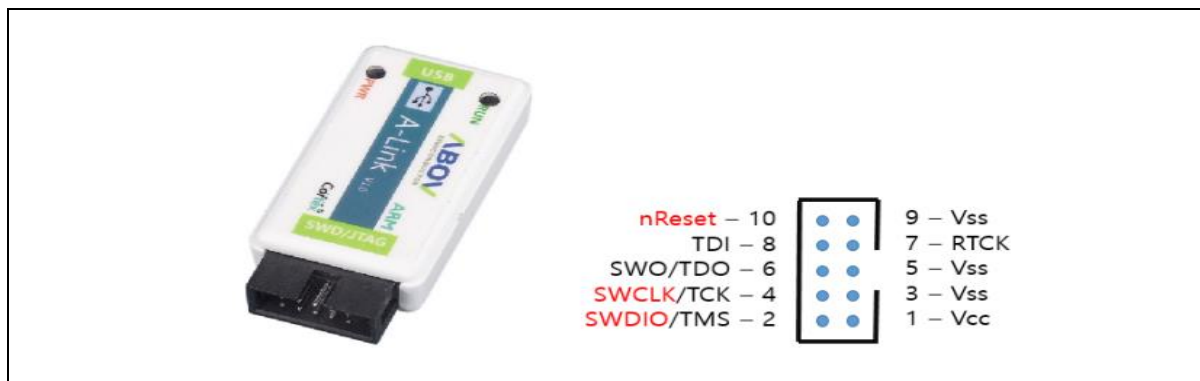
Figure 56. A-Link and Pin Descriptions
