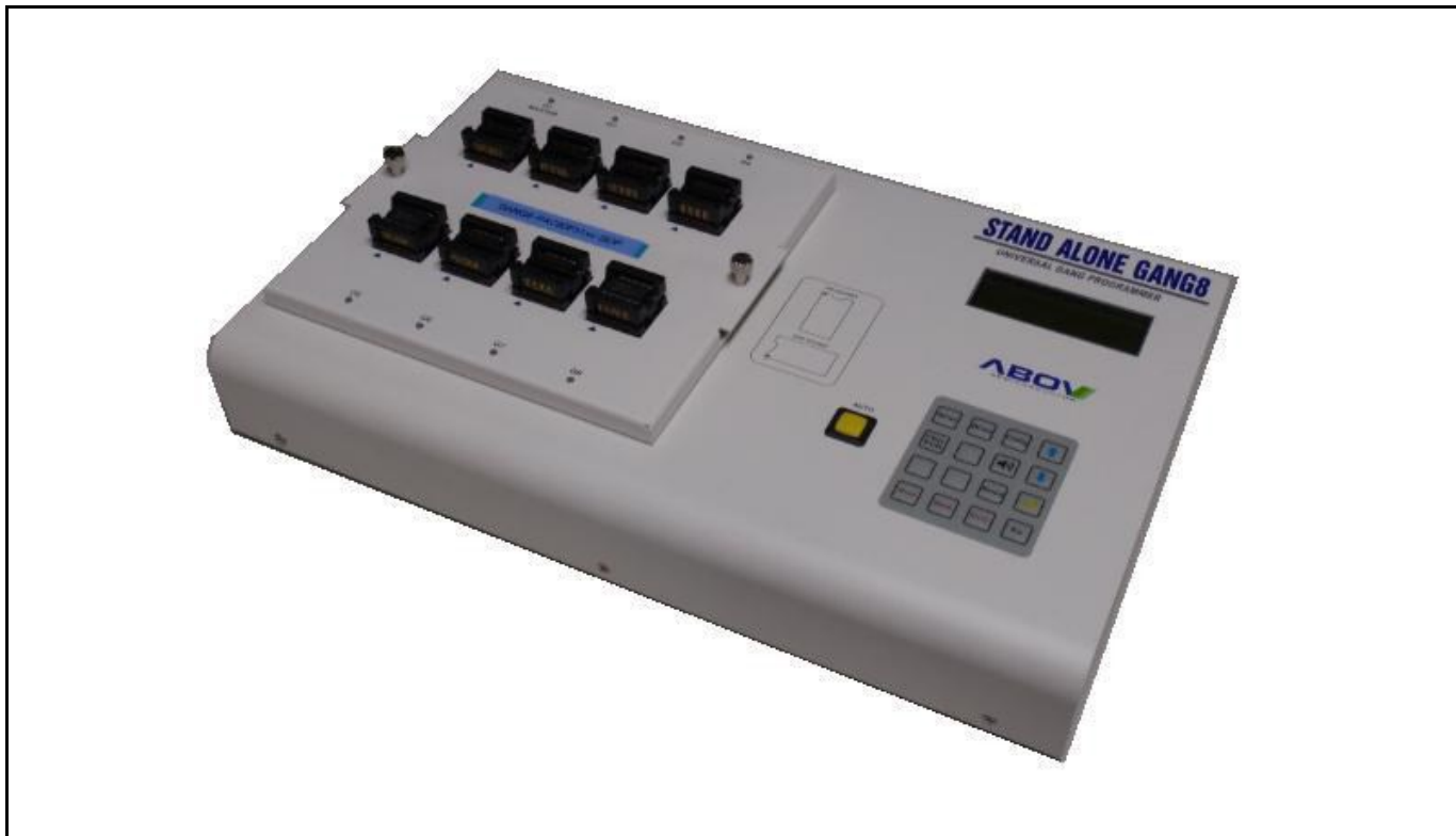
Figure 1.4 StandAlone Gang8 (for Mass Production)
