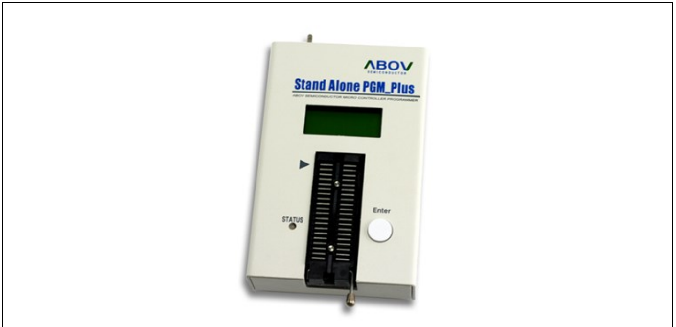
Figure 1.3 Standalone PGMplus(Single writer)
