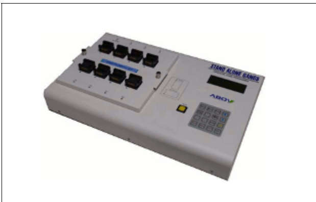
Figure 1-5 Standalone Gang8 (Gang Writer)
